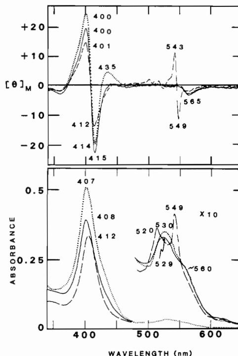
Fig. 2. MCD (upper) and absorption (lower) spectra of cyt. *c* (5  $\mu\text{M}$ ) (.....), the intermediate thiol-bound form of cyt. *c* (5  $\mu\text{M}$ ) in the presence of 1.08 mM n-propylmercaptan (—) and the reduced form of cyt. *c* (5  $\mu\text{M}$ ) in the presence of 1.33 mM n-propylmercaptan (- - -).
