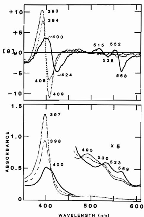
Fig. 4. MCD (upper) and absorption (lower) spectra of H8PT ( $10 \mu M$ ) (.....), the intermediate thiol-bound form of H8PT ( $10 \mu M$ ) in the presence of  $4.91 \text{ mM}$  methylmercaptan (---) and the second thiol-coordinated form of H8PT ( $10 \mu M$ ) in the presence of  $6.55 \text{ mM}$  methylmercaptan (—).
